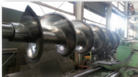
MAIN SCREW FABRICATION
